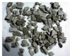
Gravel, washed 1/2" minus with some fines:
